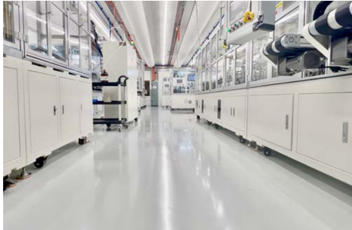
Our 220sqm dry room houses our 2MWh lithium sulfur pouch cell production facility — both the largest in Australia.
