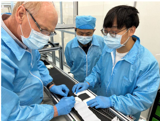
Bob Galyen (left) discusses cell stacking with our production team in the 2MWh cell fabrication Dry Room in Geelong.
