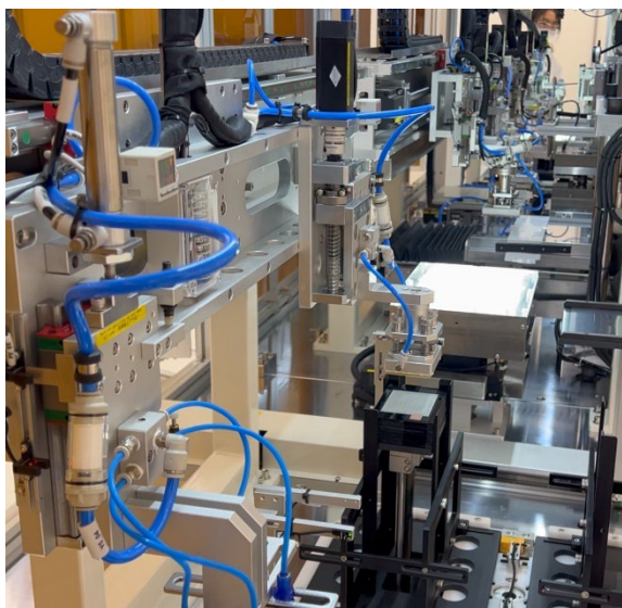
2. Robotic systems inside the automated lithium metal anode cutter
