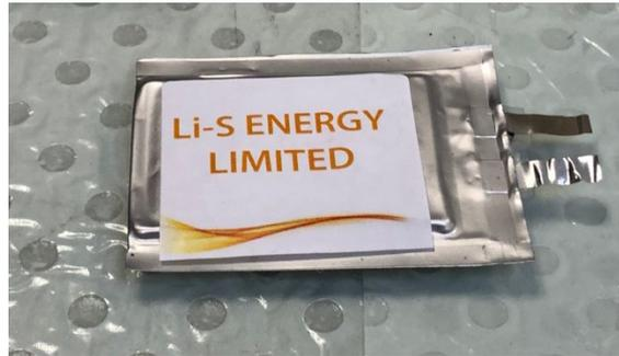
*Images above show an Insitu Pacific small UAS during flight preparation, and Li-S Energy multi-layer lithium sulphur pouch cell that will be scaled up during the project to meet UAS requirements.*
